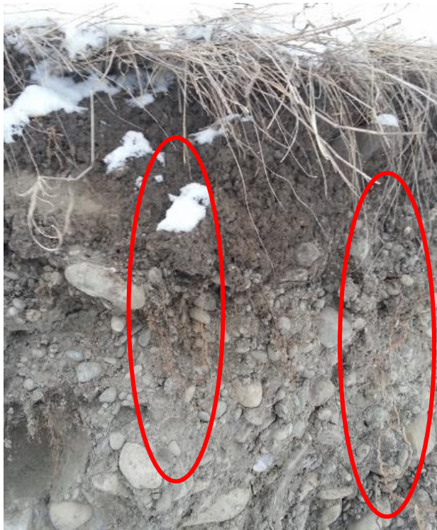
Figure 1. Root development at depth, mechanically attaching topsoil to subsoil
